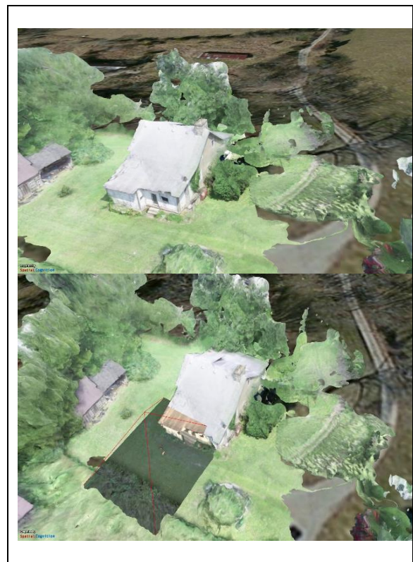
Figure 5. Pegasus 3D mapping from video (left) with "table clothing" of live video over the 3D map for change detection.
